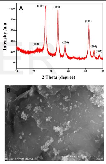
Fig.1(A) XRD pattern of SnO2@Gr (B) FE-SEM image of SnO2@Gr.
